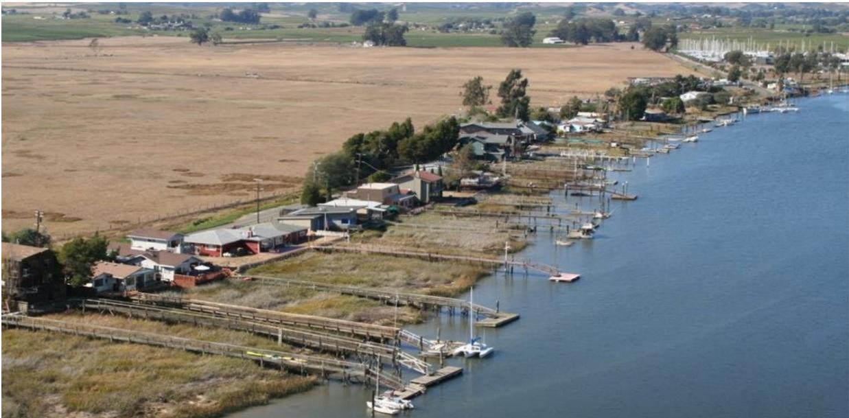
Note that at low tide most sections of the levee are only 2-3 feet above the river; they are much less at high tide.
