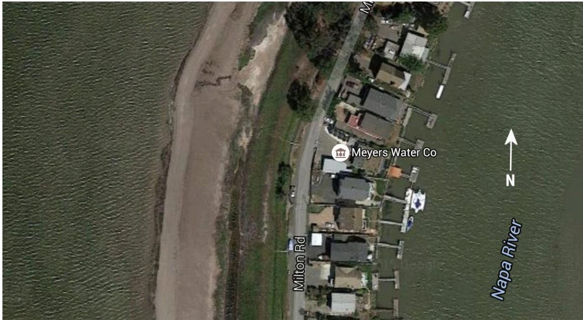
High tide waters push into the slough on the west side of the development; there is only a partial levee protecting the west side. The Napa River abuts against the levee on the east side.
